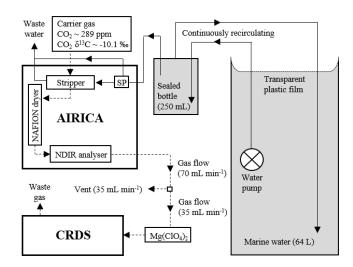
Figure 1. Schematic of the coupled Autonomous Infra Red Inorganic Carbon Analyser (AIRICA) and Cavity Ring Down Spectrometer (CRDS) set up to autonomously and continuously measure DIC concentrations and  $\delta^{13}$ C-DIC values. Solid arrows indicate liquid flow and dashed arrows indicate gas flow. SP = syringe pump.
