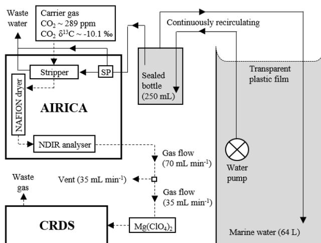
Figure 1. Schematic of the coupled Autonomous Infra Red Inorganic Carbon Analyser (AIRICA) and
