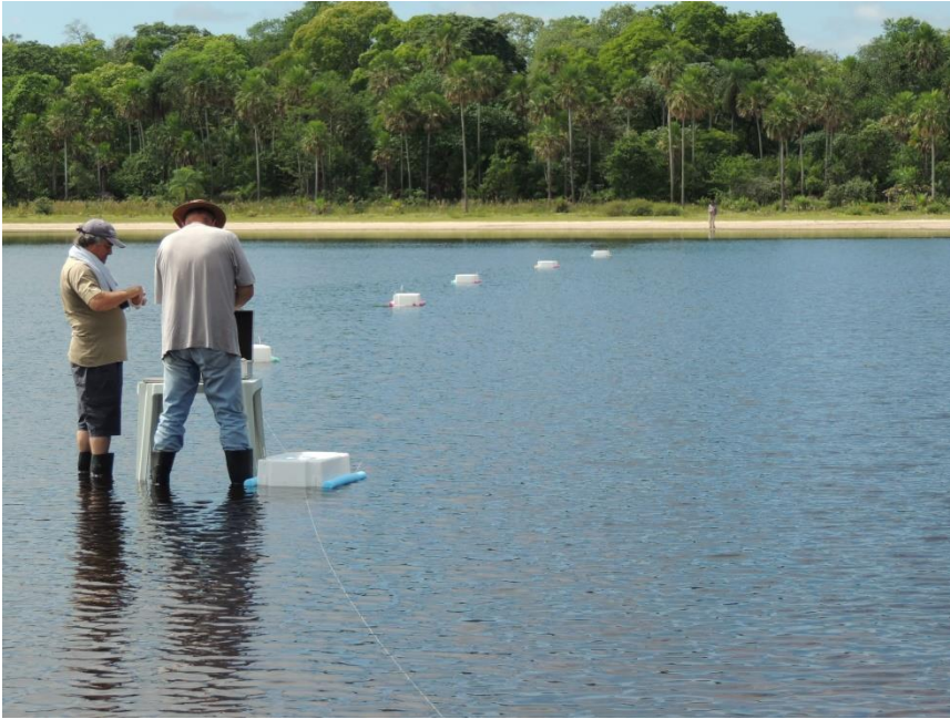
Photo 2: Gas collection from a train of 6 slowly moving chambers on green water lake M in the absence of cyanobacteria bloom (December 2014). The first floating chamber has just reached the point of collection. Two samples will be collected in each chamber. The average of these 12 samples will provide 1 flux data for each gas (CH 4 , CO 2 and N 2 O).
