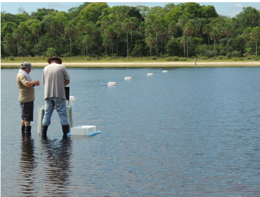
Photo 2: Gas collection from a train of 6 slowly moving chambers on green water lake M in the absence of cyanobacteria bloom (December 2014). The first floating chamber has just
