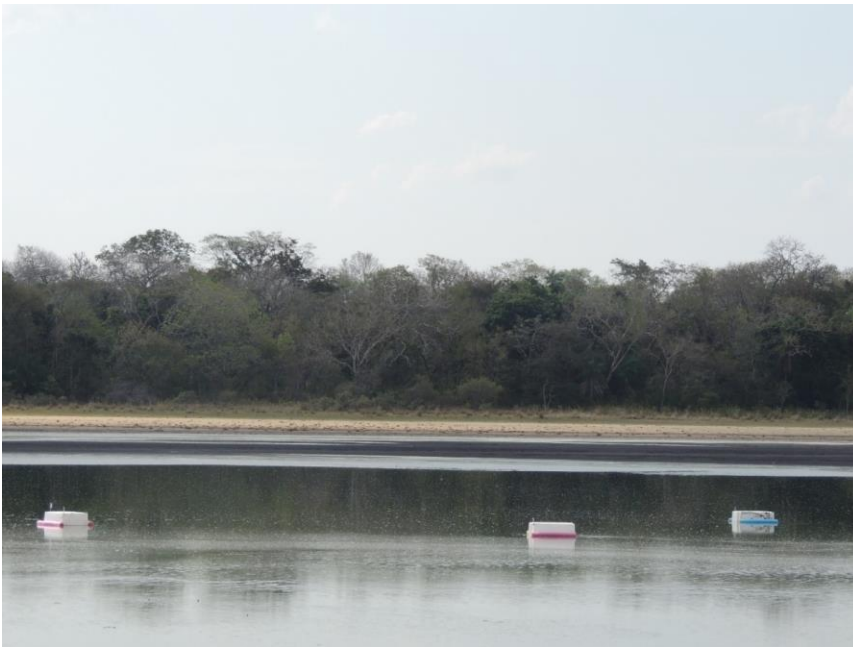
Photo 3: Gas collection from a set of 3 fixed floating chambers on Lake G with strong bloom condition (September 10, 2015). Two samples will be collected in each chamber after 20 min. The average of these 6 samples will provide 1 flux data for each gas (CH 4 , CO 2 and N 2 O). Note that the ebullition of the lake due to O 2 -supresaturation has started.
