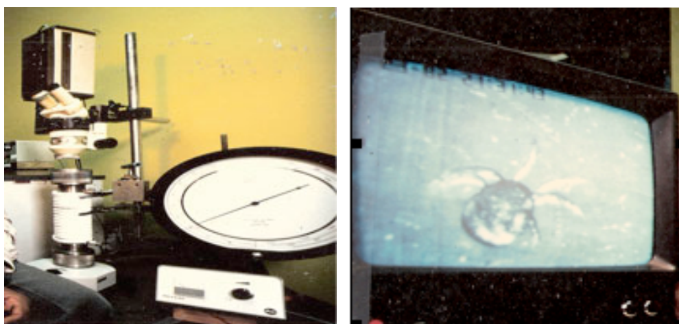
Fig. 5. left – Pressure chamber outfitted with Right - Newly hatched nauplius larva Microscope to observe krill egg development at 100 atm in a simulated sinking with a TV camera to videotape different rate in the laboratory in Palmer, stages such as blastulation, gastrulation and limb-bud formation.
