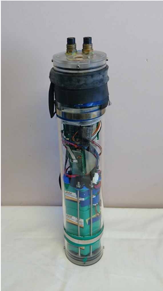
395 Figure 2. Submersible logging pH monitor. The fluorescence spot is located on the upper faceplate between and forward of the two submersible connectors, beneath a clear plastic ring.
