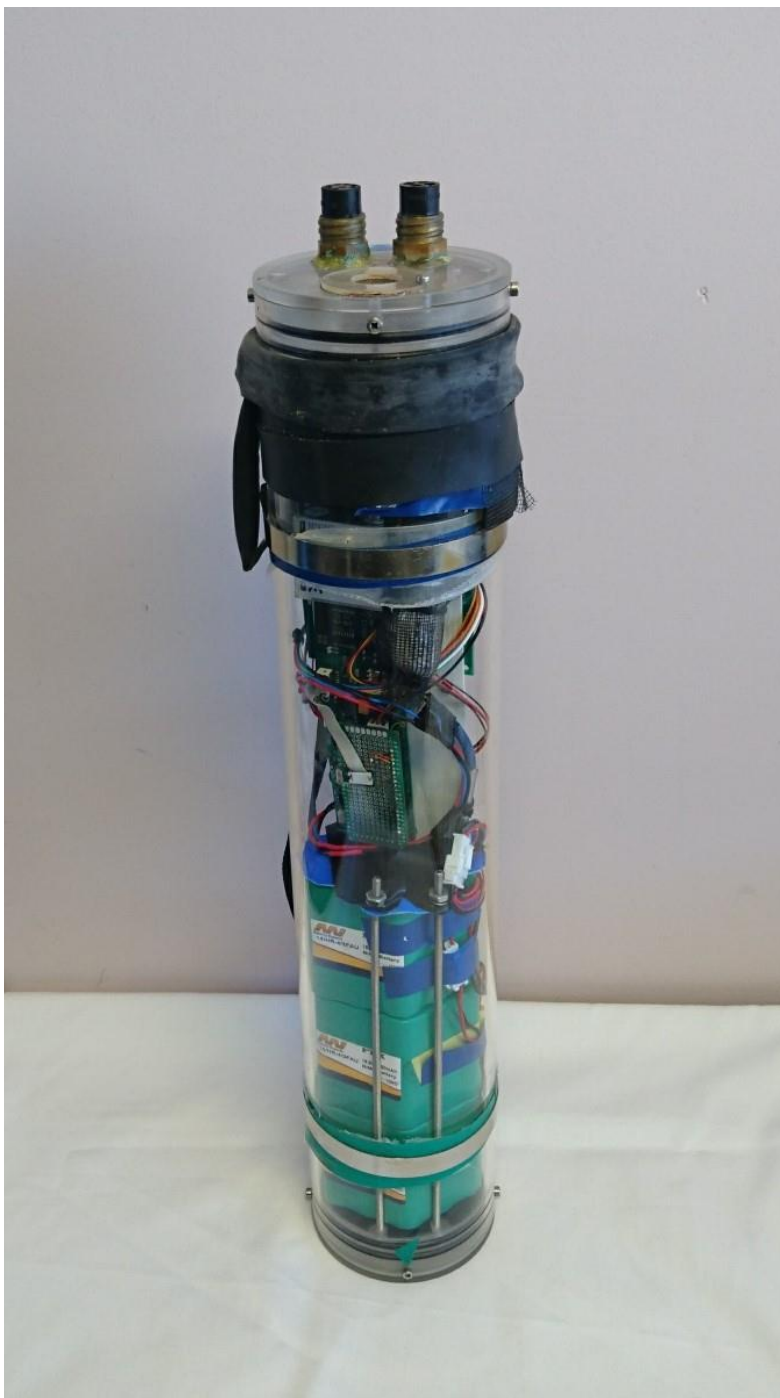
315 Figure 2. Submersible logging pH monitor. The fluorescence spot is located on the upper faceplate between and forward of the two submersible connectors, beneath a clear plastic ring.
