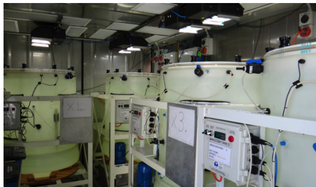
Figure 1. Minicosm tanks filled with seawater in temperature controlled shipping container.
