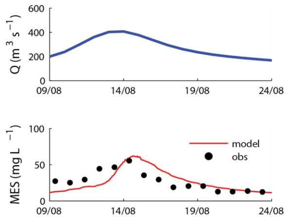
Figure A6. Discharge and observed and modeled TSS concentration during the selected storm event.
