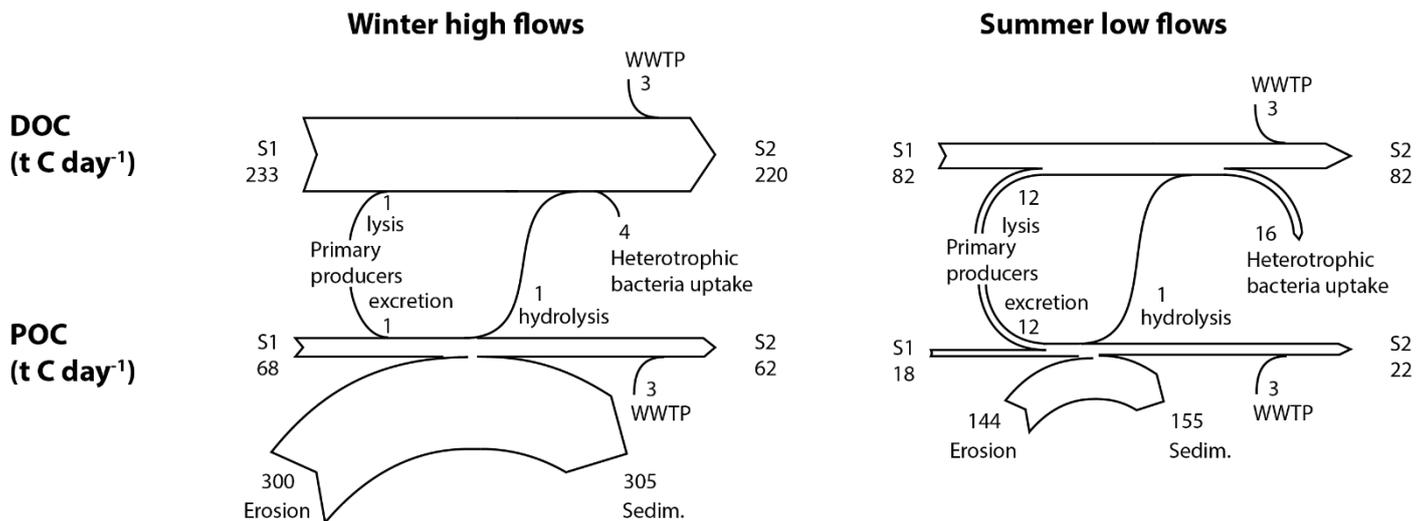
Figure A4. DOC and POC budgets assessed with QUAL-NET between S1 and S2
