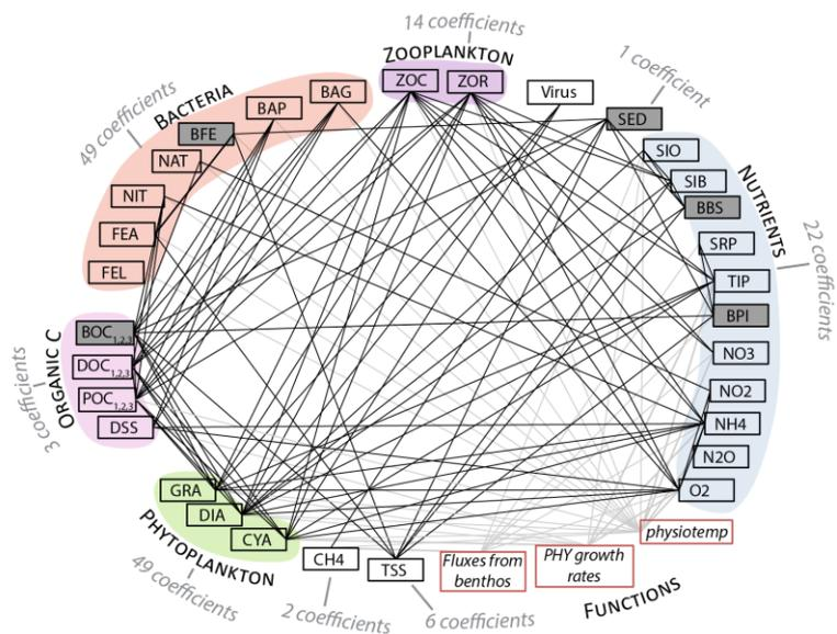
Figure 3. Main variables interdependency in the biogeochemical model RIVE and associated ~~counted~~ coefficients. Grey plain rectangles identify variables **describing** the benthos component, red rectangles are generic functions often called within the code.
