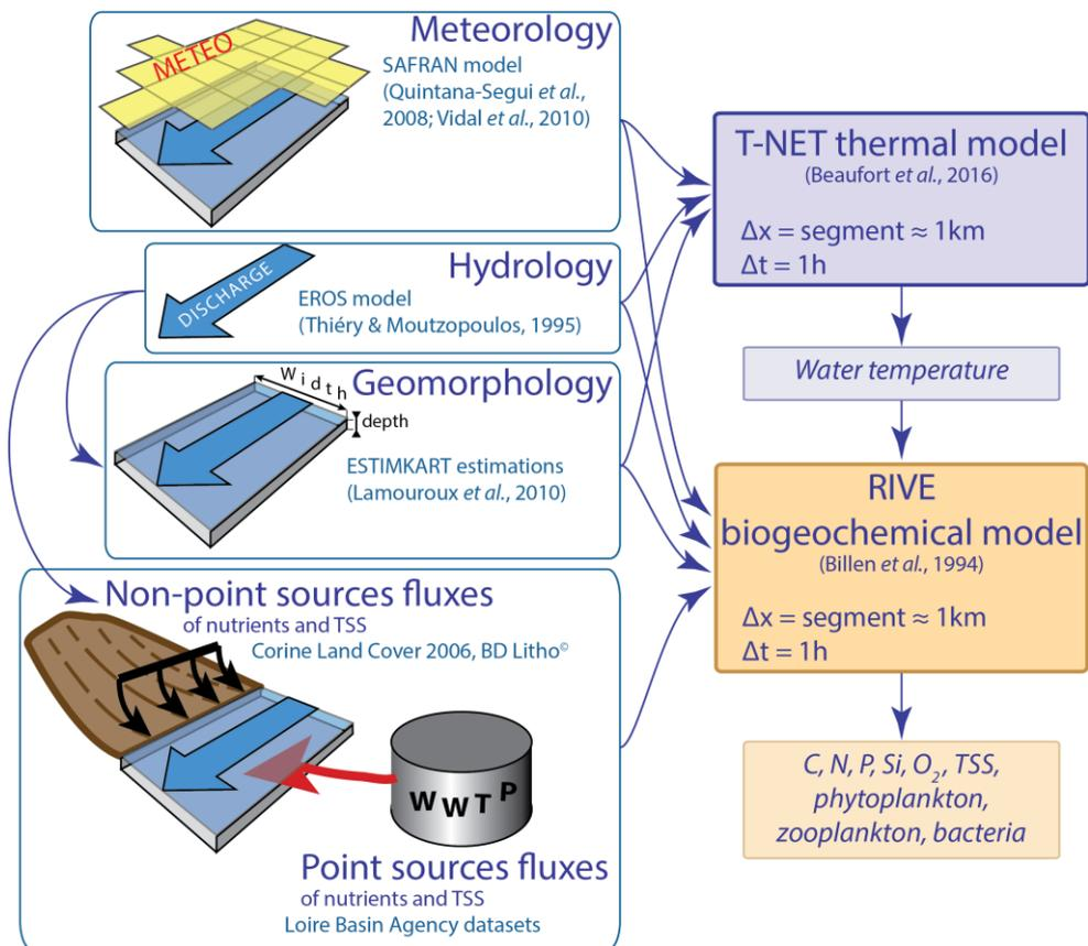
Figure 2. Architecture of QUAL-NET and [data sources](#) for the different types of forcing variables.
