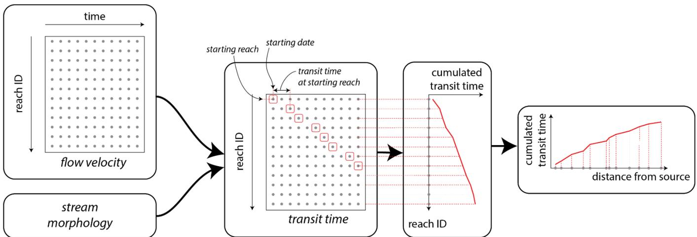
Figure A5. Successive steps to produce Lagrangian longitudinal profiles
