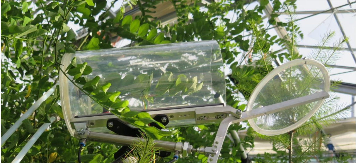
Fig S3: Picture of a leaf chamber enclosing a black locust leaf. The lid closed automatically during measurements for about 10 minutes. Between measurements the lid remained open and a fan was circulating air constantly.
