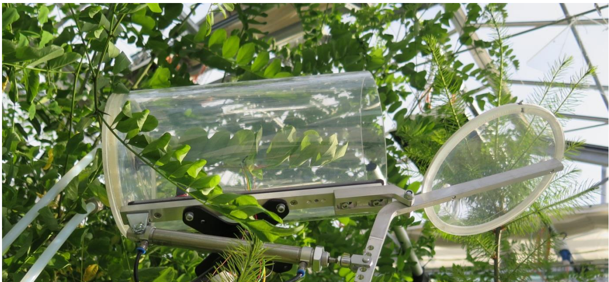
Fig S3: Picture of a leaf chamber enclosing a black locust leaf. The lid closed automatically during measurements for about 10 minutes. Between measurements the lid remained open and a fan was circulating air constantly.
