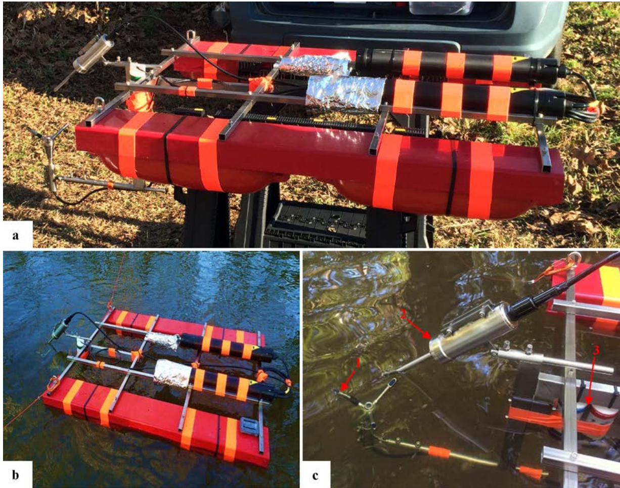
Figure 1: Floating platform for determining air-water gas exchange. (a) The 1.2 \times 0.9 m wide platform with a catamaran-shaped hull being prepared for deployment. Four inflatable fenders provide flotation. (b) The platform deployed in the Hardware River and anchored to both river banks. A dive weight is used to level the platform. (c) Close-up look at: 1) the three-pronged upward-facing sensor head of the cabled Acoustic Doppler Velocimeter (cabled Vector, Nortek AS, Norway), 2) the fast-responding dual O_2 -temperature sensor (RINKO EC, JFE Advantech, Japan), and 3) Two stable independent dual O_2 -temperature sensors used for calibration (miniDOT, PME, USA).
