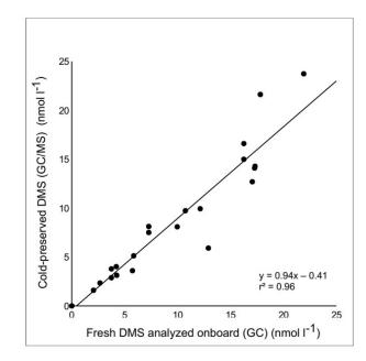
Figure 2: Relationship between the concentrations of fresh DMS samples measured on board the ship via gas chromatography during the campaign and the concentrations of the corresponding preserved duplicate samples measured via coupled gas chromatography and mass spectrometry in a laboratory setting. The concentrations of the preserved DMS samples plotted are the sum of the three isotopes of DMS investigated in this study (m/z of 62, 63, and 68; see Materials and Methods).
