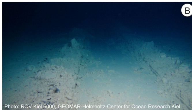
Figure A3. A) The Epibenthic sledge that created the monitored sediment plume (Photo: A. Hilario) (Brenke, 2005). B) Track created by the EBS at the seafloor, approximately 20 cm deep and 1.5 m wide Photo: ROV Kiel 6000, GEOMAR Helmholtz-Center for Ocean Research Kiel.
