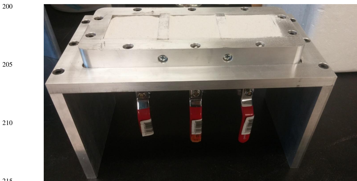
Fig. 1. Aluminum model constructed for cementation testing
