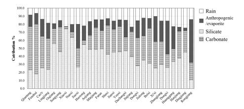
Fig. 4. Calculated contributions (in %) from the different reservoirs to the total cationic load for major rivers and their main tributaries in the SECRB. The cationic load is equal to the sum of Na<sup>+</sup>, K<sup>+</sup>, Ca<sup>2+</sup> and Mg<sup>2+</sup> from the different reservoirs.
