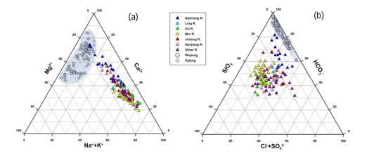
Fig. 2. Ternary diagrams showing cations (a), anions and dissolved SiO<sub>2</sub> (b) compositions of river waters in the SECRB. Chemical compositions from case studies of rivers draining carbonate rocks are also shown for comparison (data from Han and Liu 2004; Xu and Liu 2007, 2010)
