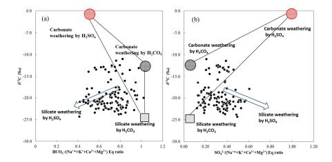
Fig. 7.  $\delta^{13}C_{DIC}$  vs. HCO<sub>3</sub>/(Na\*+K+Ca+Mg) (a) and SO<sub>4</sub>/(Na\*+K+Ca+Mg) Eq ratio (b) in river waters draining the SECRB. The plot show that most waters deviate from the three endmember mixing area (carbonate weathering by carbonic acid and sulfuric acid and silicate weathering by carbonic acid), illustrating the effect of sulfuric acid on silicate weathering.
