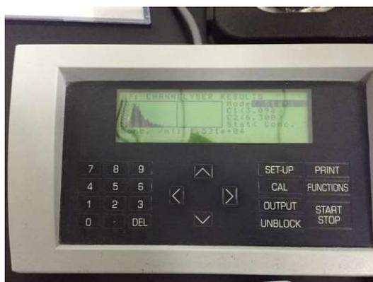
Figure R3 Cell concentration shown by a Z2 Coulter Particle Count and Size Analyzer
