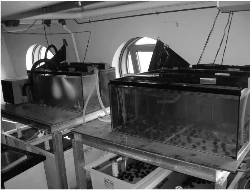
Figure 5. Experimental tank layout in Ocean Sciences Center at Logy Bay, NF. High light right end of each tank is adjacent to large port-like window and has fluorescent lights overlying. Opposite, low light ends of tanks shielded with opaque plastic sheet. Note cooling probes, coated with ice, placed in 2 & 4°C tanks on left. Three light segments (low light ll; mid light ml; high light hl, left to right) with their emplaced specimens can be seen in right tank.
