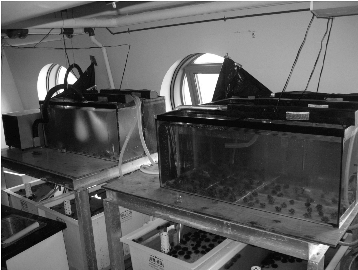
Figure 5. Experimental tank layout in Ocean Sciences Center at Logy Bay, NF. High light right end of each tank is adjacent to large port-like window and has fluorescent lights overlying. Opposite, low light ends of tanks shielded with opaque plastic sheet. Note cooling probes, coated with ice, placed in 2 & 4°C tanks on left. Three light segments (low light ll; mid light ml; high light hl, left to right) with their emplaced specimens can be seen in right tank.
