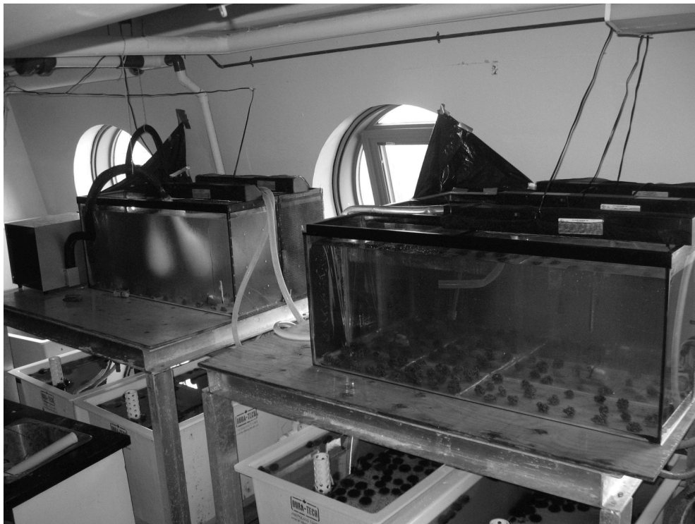
Figure 6. Experimental tank layout in Ocean Sciences Center at Logy Bay, NF. High light right end of each tank is adjacent to large port-like window and has fluorescent lights overlying. Opposite, low light ends of tanks shielded with opaque plastic sheet. Note cooling probes, coated with ice, placed in 2 & 4°C tanks on left. Three light segments (low light ll; mid light ml; high light hl, left to right) with their emplaced specimens can be seen in right tank.
