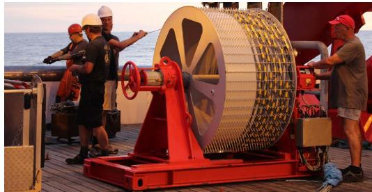
**Fig. A1**. Photo of thermistor string deployment using the instrumented cable spooling drum onboard R/V Sonne.
