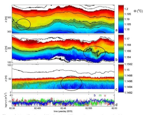
**Figure 4**. Magnifications of Fig. 3a using different colour ranges but maintaining the 5 mK distance between isotherms. (a) Upper 100 m. (b) Approximately middle 100 m. (c) Bottom 100 m; note the entire colour range extending over 1 mK only. (d) Time series of logarithm of vertical-mean turbulence dissipation rates from Fig. 3d for the panels a,b,c labelled u,m,b, respectively.
