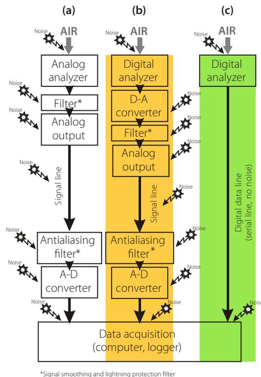
**Fig. 1.** Three variants of data acquisition systems. Modified after Eugster and Plüss (2010).
