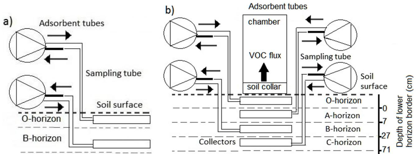
**Figure 1: Measurement set-up for soil VOC concentration profiles a) in 2008- 2011 and b) in 2016.**
