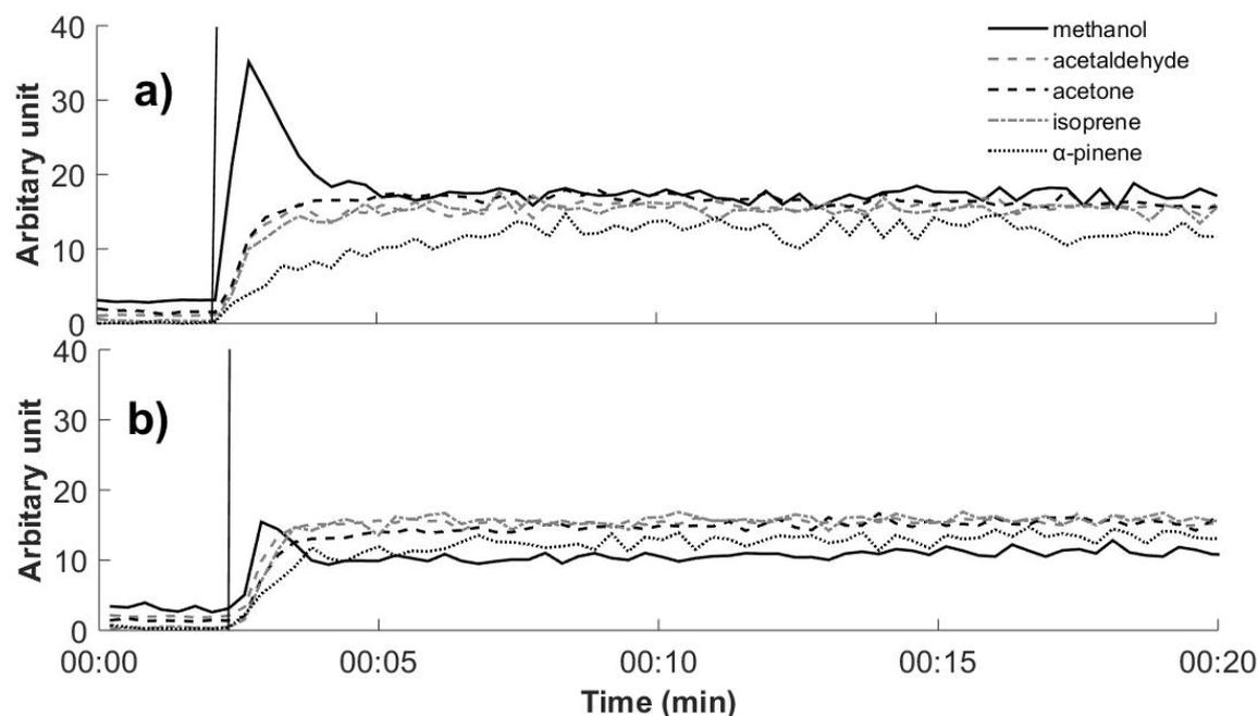
Figure 3: Results of the permeability tests of the PTFE collector with the five VOCs. A permeability test was used to monitor how fast VOCs permeate into the gas collector and to determine how fast VOC concentrations stabilize between the air inside and outside the collector. Panel a) shows the results with dry collector and panel b) with a wetted collector. Vertical line shows the time point when the introduction of the VOC standard began.
