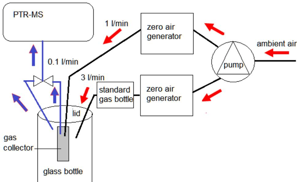
Figure 12: Set-up for the permeability tests of the sintered gas collectors. The sintered gas collector means that PTFE tube is closed on one side.
