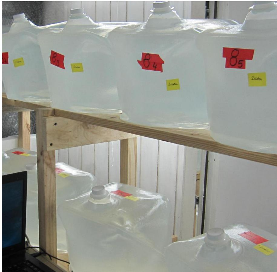
20 L containers for the multistressor experiment (one container per sampling day) were incubated on custom made racks designed to ensure equal distribution of light and to facilitate easy access to the containers for mixing/sampling (*Patagonia multistressor room shown*).
