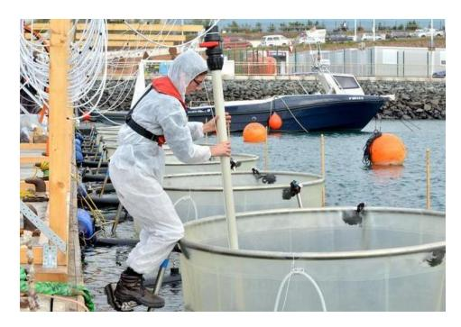
Polyurethane bags, supported by steel framework, were tethered to a jetty in Taliarte. During sampling the mesocosms were pulled adjacent to the jetty (as shown), otherwise the mesocosms were free to float 2-3 m away from the jetty.
