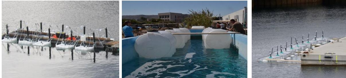
Large HDPE containers were incubated at ambient seawater temperatures tethered to jetties or, (for MesoMed) within a pool facility continuously flushed with seawater. *Left MesoArc, centre MesoMed, right MesoArc.*
