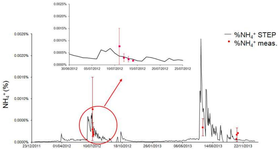
10 **Figure 6: Daily ammonium simulated by STEP-GENDEC (% , black line) and daily averaged ammonium measurement (red squares) during the field campaigns. Error bars in red give the standard deviation at the daily scale for measurements. The upper panel is a focus of J12.**
