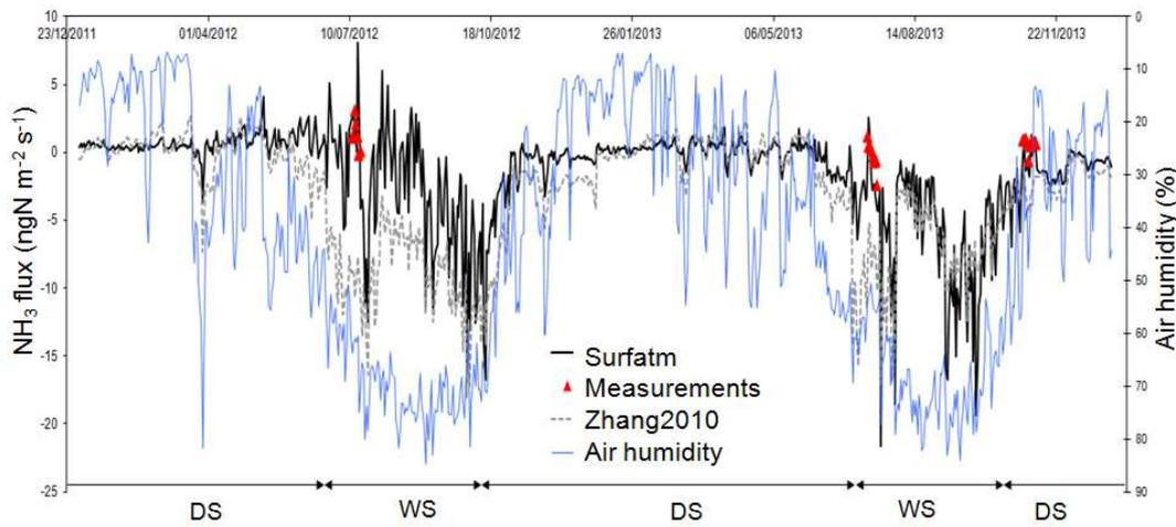
Figure 9: Daily  $\text{NH}_3$  flux (in  $\text{ngN m}^{-2} \text{s}^{-1}$ ) simulated by SurfAtm (black line) and Zhang2010 (grey dashed line) and daily averaged  $\text{NH}_3$  flux measurements during 3 field campaigns (red triangles). Error bars in red stand for standard deviation at the daily scale. Air humidity in % (blue line). DS = Dry Season; WS = West Season.
