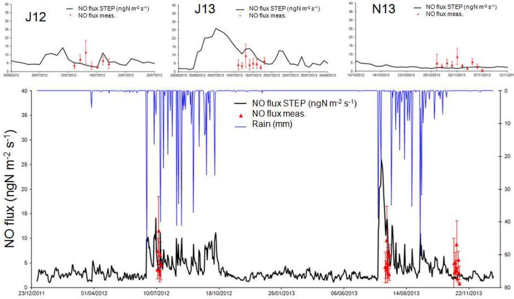
5 | Figure 5: Daily NO flux simulated by STEP-GENDEC-NOFlux ( $\text{ngN m}^{-2} \text{s}^{-1}$ , black line) and daily averaged NO flux measurements during the 3 field campaigns (red triangles). Error bars in red give the standard deviation for measurements at the daily scale. Rain is represented by the blue line in mm in the bottom panel. Upper panels give a focus on each field campaign.
