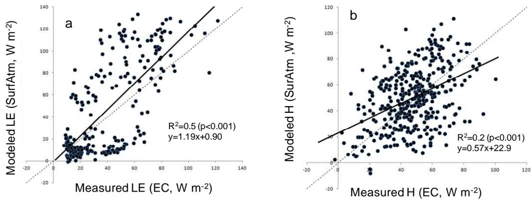
5 **Figure 3: a) Daily modelled latent heat flux in SurfAtm vs daily measured latent heat flux, in W m<sup>-2</sup>; b) Daily modelled sensible heat flux in SurfAtm vs daily measured sensible heat flux, in W m<sup>-2</sup>. Thick black line is for the linear regression, dashed black line is the 1:1 line. Available measured EC data are more numerous for H than for LE due to the criteria applied by the postprocessing (see supplementary material of Tagesson et al. (2015b)).**
