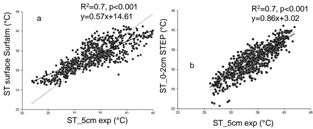
5 **Figure 4:** a) Modelled daily surface temperature in SurfAtm vs measured daily temperature at 5cm depth; b) Modelled daily surface temperature in STEP (0-2cm layer) vs measured daily temperature at 5cm depth. Thick black line is for the linear regression, dashed black line is the 1:1 line.
