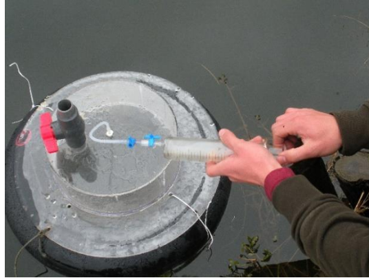
Fig. 2 The gas collection chamber for gas fluxes across the air-water interfaces in our previous studies
