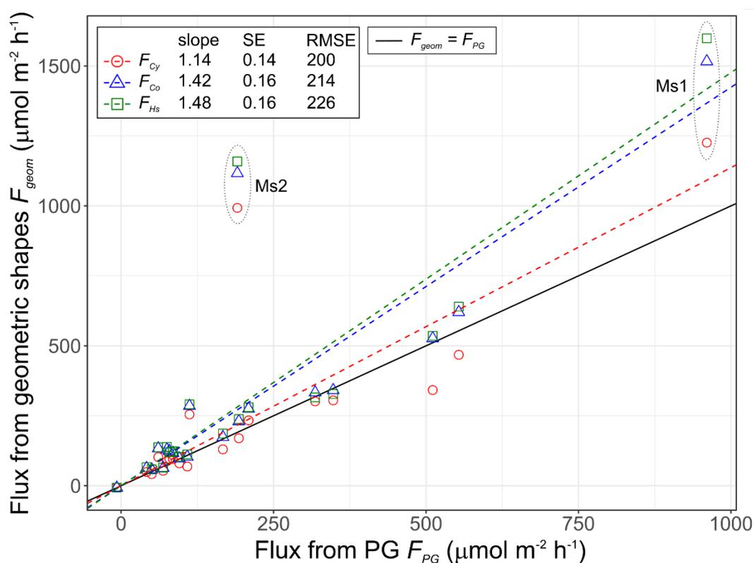
10 Fig. 6: Comparison of  $\text{CH}_4$  flux calculated according to Eq. 1 with TM epigeal volumes  $V_{TM}$  and basal areas  $A_B$  from photogrammetry ( $F_{PG}$ ), and with TM volumes approximated by three geometric shapes, a cylinder ( $F_{Cy}$ ), a cone ( $F_{Co}$ ) and a hemi-spheroid ( $F_{Hs}$ ). Considering PG as the reference method, fluxes were overestimated by  $14 \pm 14$  % for the cylinder,  $42 \pm 16$  % for the cone and  $48 \pm 16$  % for the hemi-spheroid.
