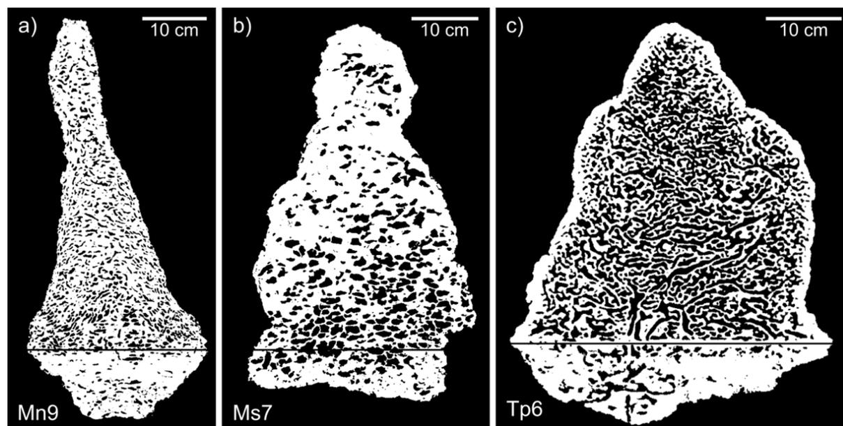
15 **Fig. 4:** Binary image of a single CT slice in xz-direction for each investigated species: a) *Microcerotermes nervosus*; b) *Macrognathotermes* spp.; c) *Tumulitermes pastinator*. The thin black line approximately indicates the soil surface.
