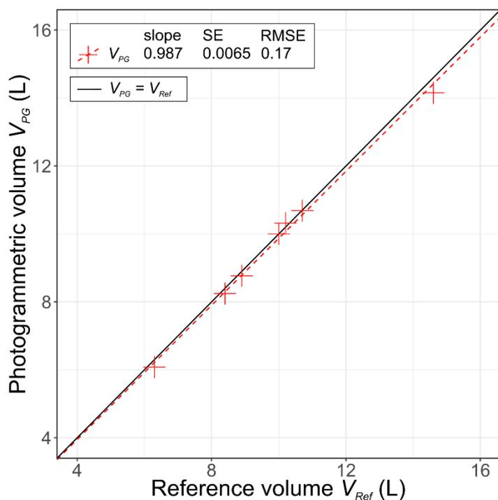
**Fig. 2: Validation of the photogrammetry method (PG) by estimating the volumes of seven irregularly shaped rocks with similar volumes to small termite mounds. The dashed line indicates the linear regression between  $V_{PG}$  and  $V_{Ref}$ ; with slope, standard error (SE) and root mean square error (RMSE); the black solid line denotes perfect correlation.**
