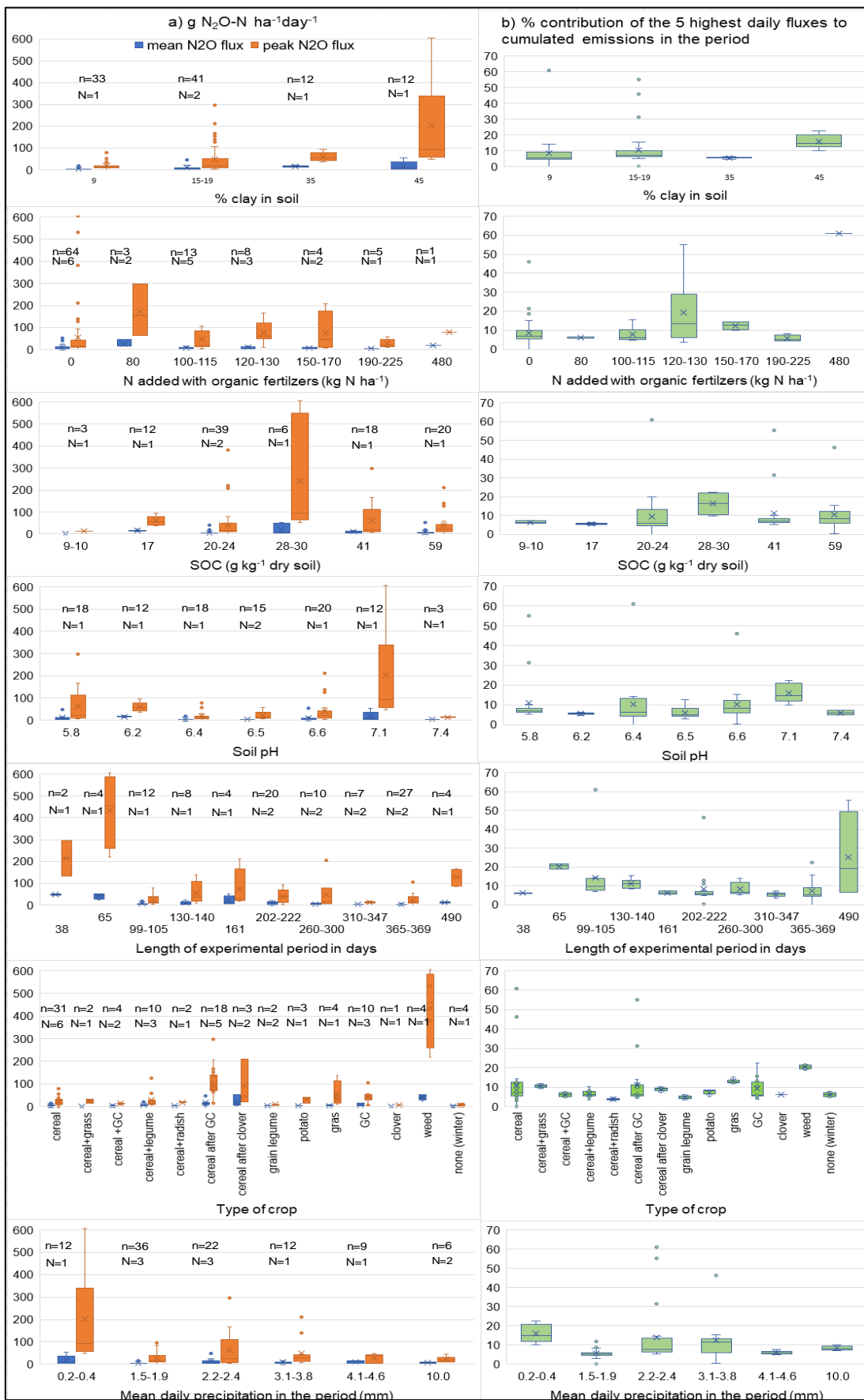
Fig.2. Box-plot (mean -, median x, upper and lower quartile) for (a) mean N 2 O flux in the period (g N 2 O-N ha -1 day -1 ) and the highest daily flux rate in the same period (g N 2 O-N ha -1 day -1 ) and (b) % contribution of the 5 highest daily fluxes to cumulated N 2 O emissions in the period. N=number of sites, n=number of observations
