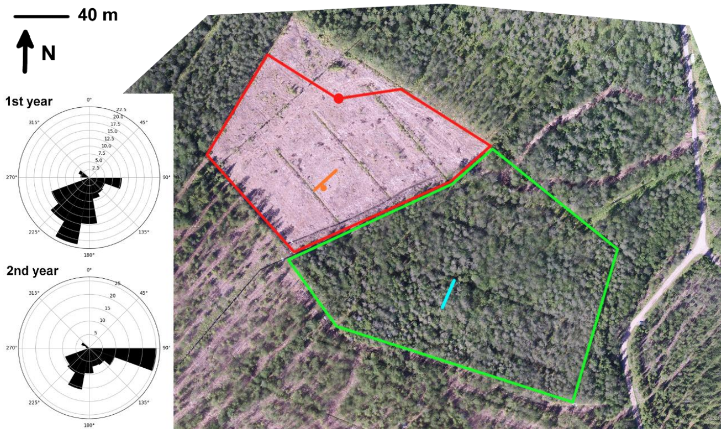
Figure 1. Aerial view of the clear-cut site and the surrounding forest at Lettosuo. The red dot shows the location of the eddy covariance mast, and the red lines surround the target area ( 80^{\circ} - 315^{\circ} ). The meteorological measurements were conducted at the location indicated by the orange dot, while the orange line marks the water table, soil temperature and chamber measurements (4, 8, 12 and 22.5 m from the ditch). Similar measurements of greenhouse gas fluxes , water table and soil temperature within the control site, surrounded by the green lines , are shown with a light blue line. The windroses on the left show the cumulative footprint contributions (in %) of the accepted flux data.
