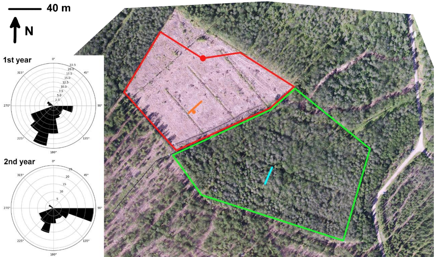
Figure 1. Aerial view of the clear-cut site and the surrounding forest at Lettosuo. The red dot shows the location of the eddy covariance mast, and the red lines surround the target area (80° – 315°). The meteorological measurements were conducted at the location indicated by the orange dot, while the orange line marks the water table, soil temperature and chamber measurements (4, 8, 12 and 22.5 m from the ditch). Similar measurements of greenhouse gas fluxes, water table and soil temperature within the control site, surrounded by the green lines, are shown with a light blue line. The windroses on the left show the cumulative footprint contributions (in %) of the accepted flux data.
