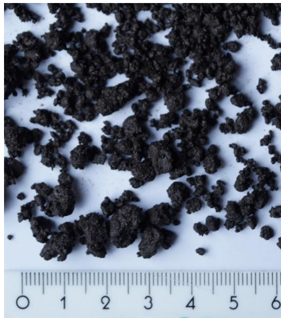
5 Figure S3 Example of the crushed nodule substrate. Scale in centimetres.
