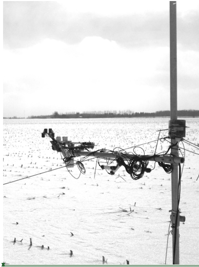
Photo S1: Silicon-based and CNR1 pyranometers measuring albedo at the Elora Research Station, Guelph, Ontario, Canada (Photo Credit: Shannon Brown, Postdoctoral Research Associate, School of Environmental Science, University of Guelph).
