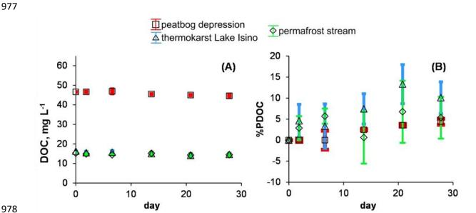
**Fig. 3.** Concentration (A) and percentage of degradable (B) DOC in photo-degradation experiments. The experiments are shown by solid symbols and the control runs are shown by open symbols: red squares, peatbog depression; green diamonds, permafrost stream; and triangles, thermokarst Lake Isino. The error bars are 1 s.d. of triplicates.
