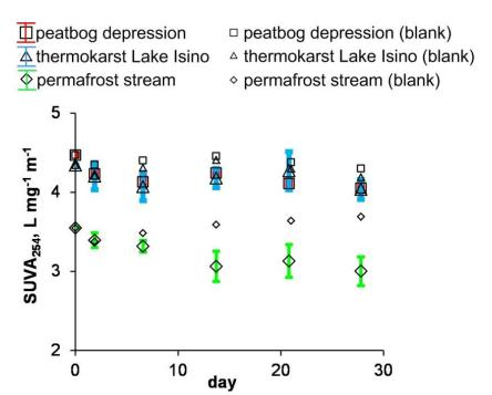
**Fig. 4.** SUVA<sub>254 nm</sub> over time in photo-degradation experiments. The error bars are 1 s.d. of triplicates.
