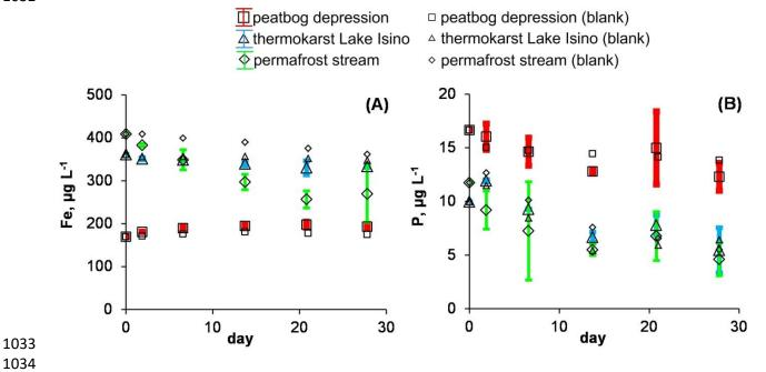
**Fig. 5.** Fe (A) and P (B) concentration over time in photo-degradation experiments. The error bars are 1 s.d. of triplicates.
