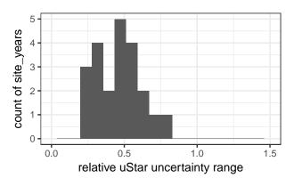
Figure C3. Histogram of ratio (REddyProc / DP06) of uncertainty ranges of uStar (90% quantile - 10% quantile). The clustering around 0.5 shows that the estimated uncertainty with REddyProc is only about half the uncertainty estimated by DP06.
