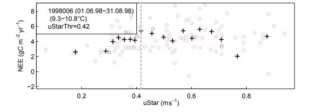
**Figure 2.** Concept of the uStar-filter: NEE at low uStar friction velocities below a threshold, i.e with low turbulence, is biased low compared higher uStar with otherwise similar environmental conditions. The uStar threshold (dashed line) is estimated by a moving point method on uStar bins (crosses) across half-hourly records (circles) here for a season-temperature subset of data from DE-Tha.
