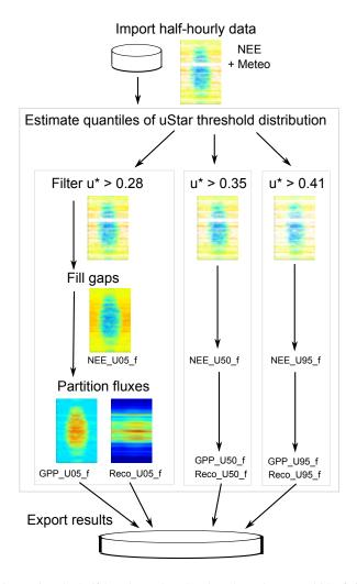
**Figure 1.** The workflow starts with importing the half-hourly (or hourly) data, here the year 1998 of site DE-Tha is plotted as an example. Next, a probability distribution of uStar threshold is estimated for each season. Gap-filling and flux-partitioning is performed for several quantiles of this distribution for an estimate of uncertainty. Finally the results are exported.
