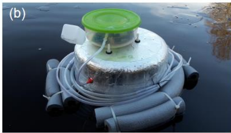
Figure 1: (a) Schematical drawing of the floating chamber with automatic ventilation showing the box, which contains air pump, timer and battery (upper part); cross-section (lower left) and view from above (lower right) of the entire floating chamber, (b) picture showing the floating chamber deployed on a lake, and (c) floating chamber viewed from above showing the exterior box containing air pump and timer.
