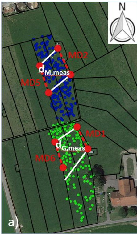
2 Figure 3: (a) GPS tagged dung positions recorded after grazing rotation 7 overlaid on a Google Earth image of the experimental 3 area (Map data: Google, DigitalGlobe). The positions of the MD ammonia sensors/paths are indicated by the red dots/dotted lines. 4 The white lines enclose the main emission measurement area between the sensors. Their dung patch density d_{x,meas} was related to 5 the average density over the investigated paddocks according to Eq. 2; (b) comparison of k_d values according to Eq. 2 for dung patch 6 and cow position distributions on system M (blue) and system G (green)
