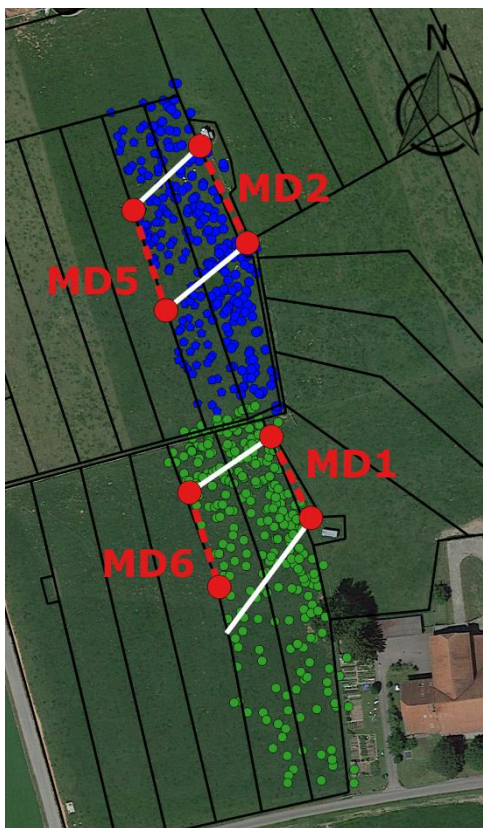
Figure 9: GPS dung positions overlaid on a Google Earth image of the experimental area (Map data: Google, DigitalGlobe). The positions of the MD devices are indicated by the red dots and the red dotted line show the light path between the MD systems and the light reflector. The white lines show the border between monitoring sections.
