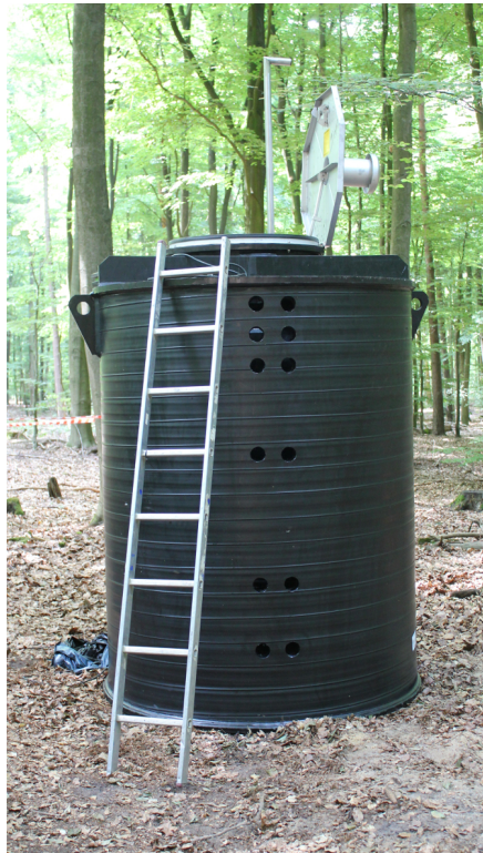
Fig. 3. Photograph of the used polyethylene shaft inserted thereafter.
