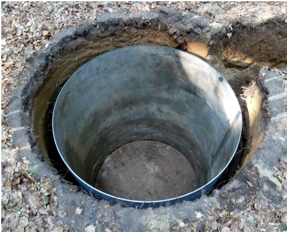
Fig. 2. Photograph of the used lysimeter vessel to drill the whole for the subsoil observatory.
