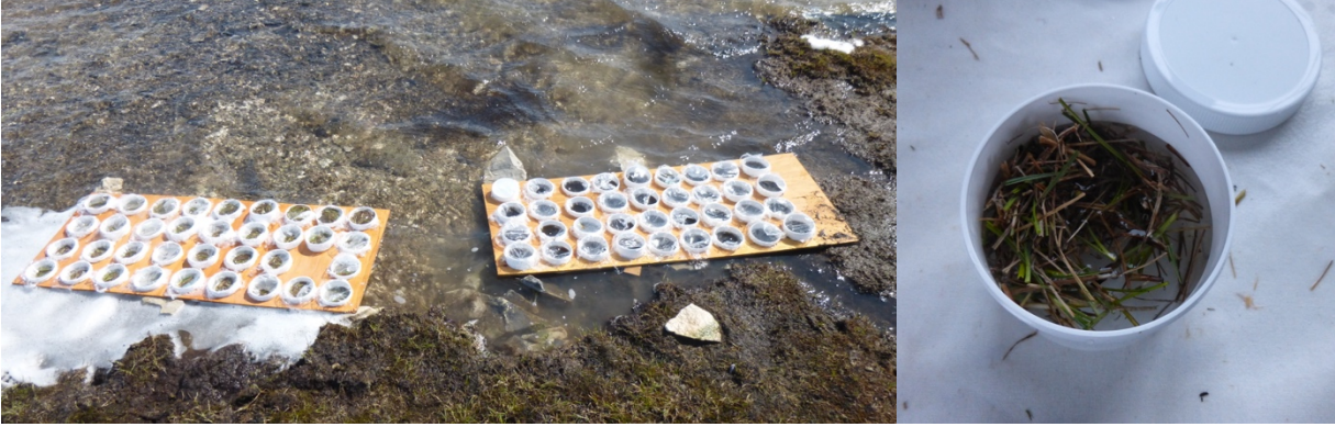
Figure 1. Mesocosm set up in the pond, sample cups had either fresh Carex clippings or fresh goose droppings submerged in 200 mL of pond water. The organic matter and the water from experimental cups were sampled throughout the 17-day experiment.
