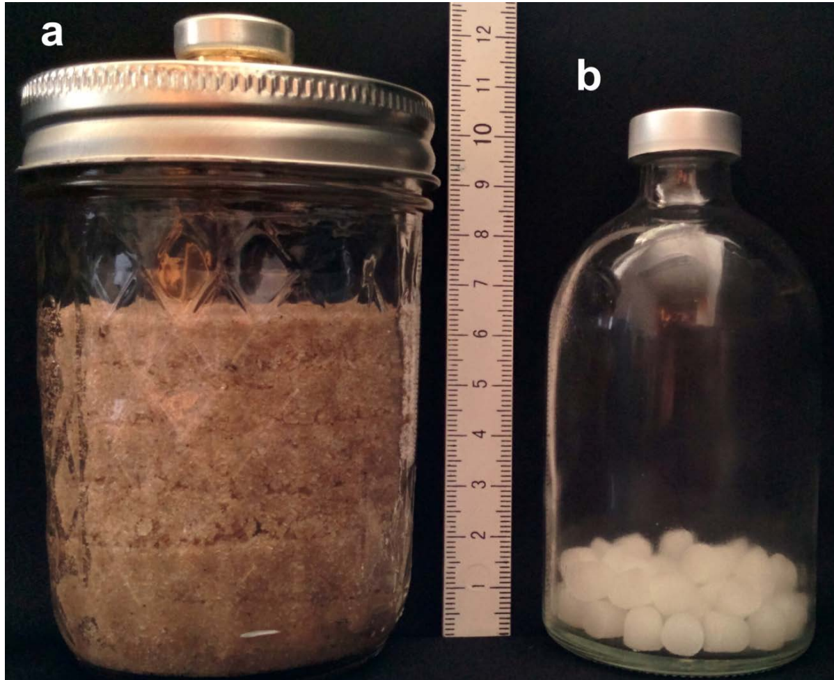
Figure S1: (a) Half-pint incubation jar (230ml) filled with sand and porous glass beads that serve as microbial hotspots. (b) Respiration kinetics of different types of hotspots either inoculated with Agrobacterium tumefaciens or Paracoccus denitrificans are measured with 50 hotspots in an otherwise empty glass jar (120ml). Note that hotspots are packed densely with minimal distance, which might have affected aeration.
