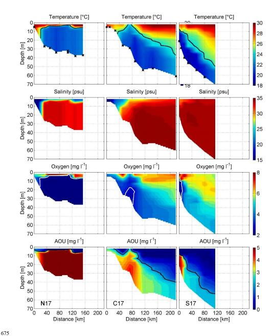
Fig. 5. Vertical distributions of temperature, salinity, density, DO concentration and AOU along sections N17, C17, S17 in 2017 (Fig. 1). Temperature isoline 24.5 °C and AOU isoline 2 mg  $\rm I^{-1}$  (upper panels) are shown with solid black line. Hypoxia border (3.0 mg  $\rm I^{-1}$ ) is shown with solid white line. Values on the *x*-axis indicate the distance from the westernmost point of a section (Fig. 1).
