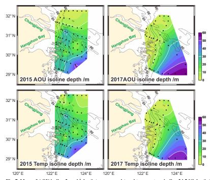
Fig. 7. Maps of AOU isoline 2 mg l $^{-1}$  depth (upper panels) and temperature isoline 24.5 °C depth (lower panels) in 2015 (left panels) and in 2017 (right panels).
