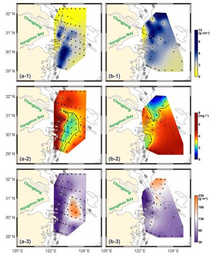
Fig 6. Maps of density difference between the near-bottom layer and surface layer (upper panel), near-bottom DO (mid-panel) and total AOU in the water column (lowest panel) in 2015 (left) and 2017 (right). Only positive values of AOU were used in the vertical integration of the AOU profile.
