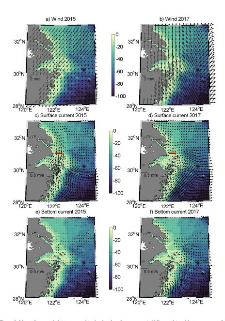
Figure 8. Maps of mean wind (upper panels), simulated surface current (middle panels) and bottom current (bottom panels) 7 days prior to the CTD surveys. Bottom bathymetry is shown as a background. Red lines show the section S1, where current time-series were calculated. Every fourth current vector is shown only. Persistent current in the southeastern side is the Taiwan Warm Current.
