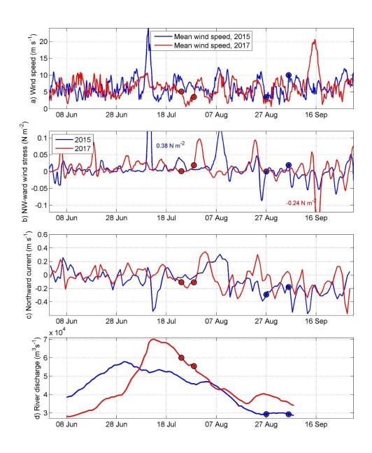
Figure 10. Time-series of wind, current, and river discharge. Mean wind speed (6-hours) (a), 1-day running mean SE-NW wind stress  $\boldsymbol{\epsilon}$  (positive towards NW; N m²) (b), daily mean meridional current velocity component  $\nu_m$  (positive northward) at section S1 (c), and daily Changjiang river discharge at Datong station shifted by 7 days to represent flow in the river mouth (d). Blue and red dots represent start and end of the CTD surveys, respectively in 2015 and 2017.
