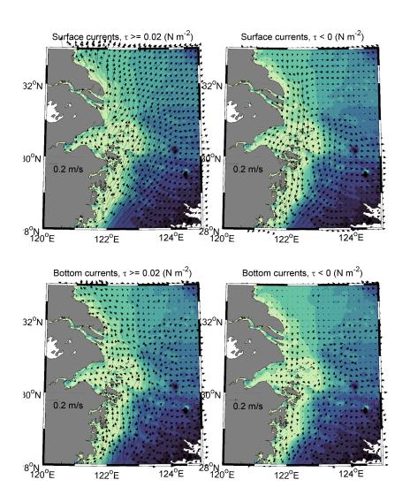
Figure 12. Maps of surface (upper panels) and near-bottom (lower panels) currents in the cases of wind stress component  $\tau_c \geq 0.02~N~m^2$  (left panels) and  $\tau_c < 0~N~m^2$  (right panels) in 1993-2018. Every fourth current vector is shown.
