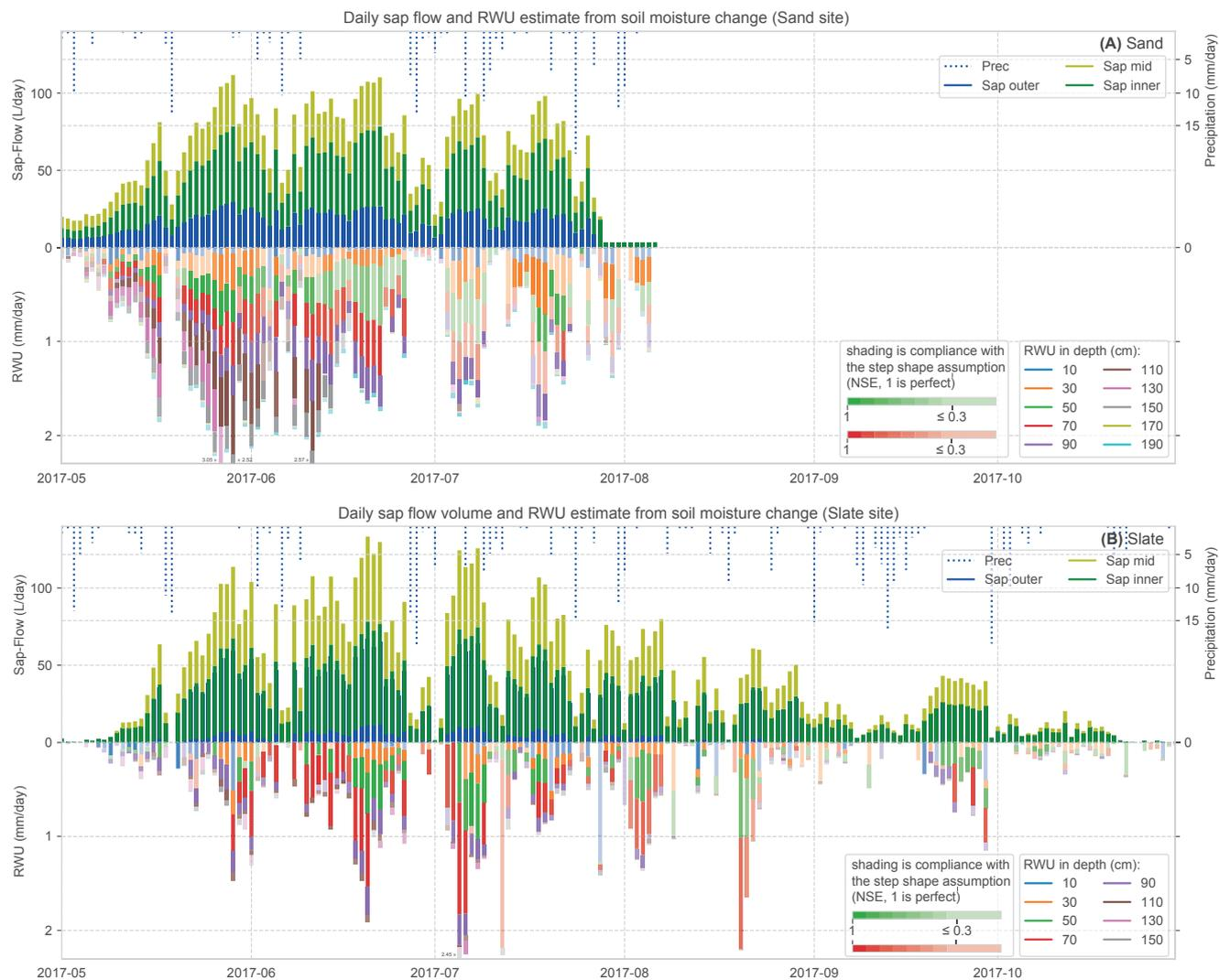
**Figure 6.** Sap flow (upper part) and RWU estimate (lower part) at two sites. The colour coding of the different depth sources of RWU is complemented with its color strength taken from the NSE evaluation of the step shape evaluation (opaque is high compliance/high NSE).
