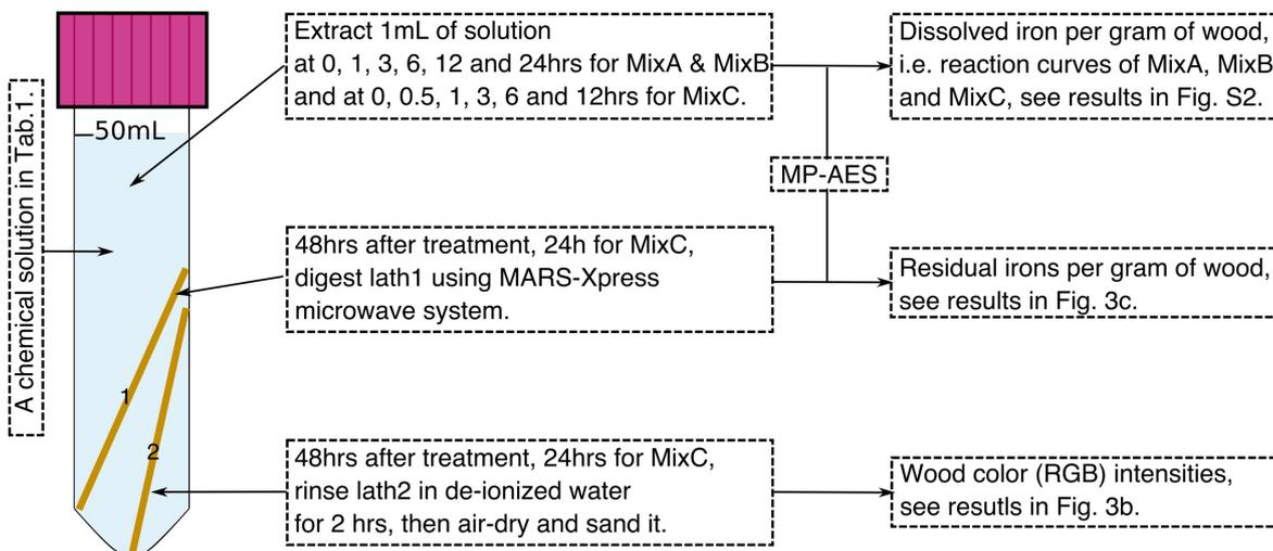
50 **Figure 2.** Diagram of one chemical de-staining experiment for one pair of wood laths from the same subfossil tree in a Falcon® 50mL tube.
