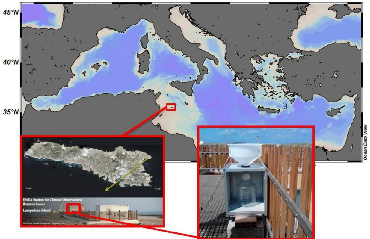
Figure 1: Sampling location (Lampedusa island 35.5° N, 12.6° E) and the total atmospheric deposition collector.
