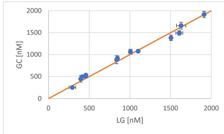
Figure 1 Average CH<sub>4</sub> concentration measured with lab-based GC method (n=2) versus field-based LG method (n=3). Error bars show the standard deviation, the orange line symbolizes the 1:1 line.
