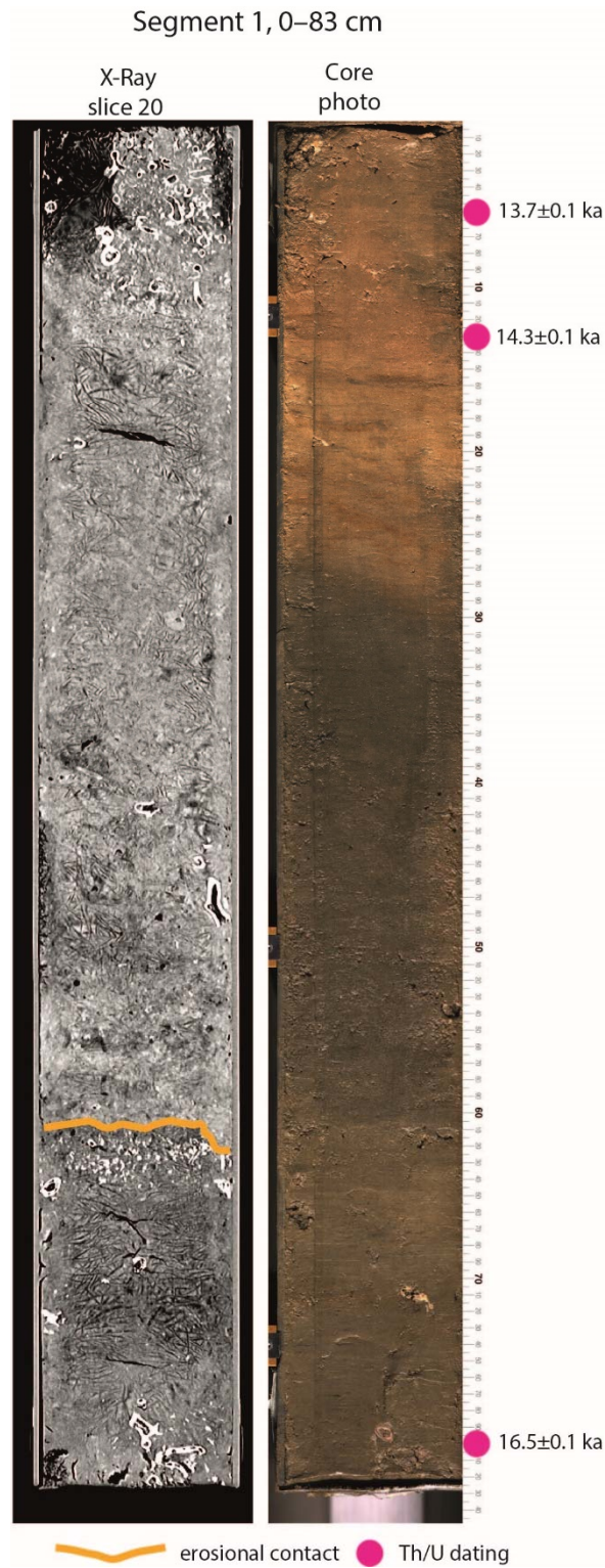
565 Appendix Figure A: CT image (left) and photography (right) of segment 0-83 cm of core M125-34-2. Erosional contacts are marked by thick black lines, position of Th/U datings with calibrated ages are indicated by magenta dots.
