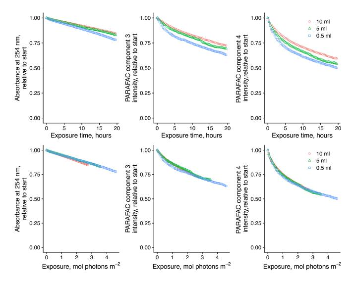
Figure 3. Photodegradation time series of absorbance at 254 nm and fluorescence intensities of PARAFAC component 3 and 4 relative to starting values. Data are shown from experiments with SRNOM PPL that varied volume of sample added to mixing reactor (after filling flow cell lines). Top panels show values as a function of exposure time, while bottom panels show values as a function of cumulative photon exposure calculated from NO<sub>2</sub>/NO<sub>3</sub> actinometry.
