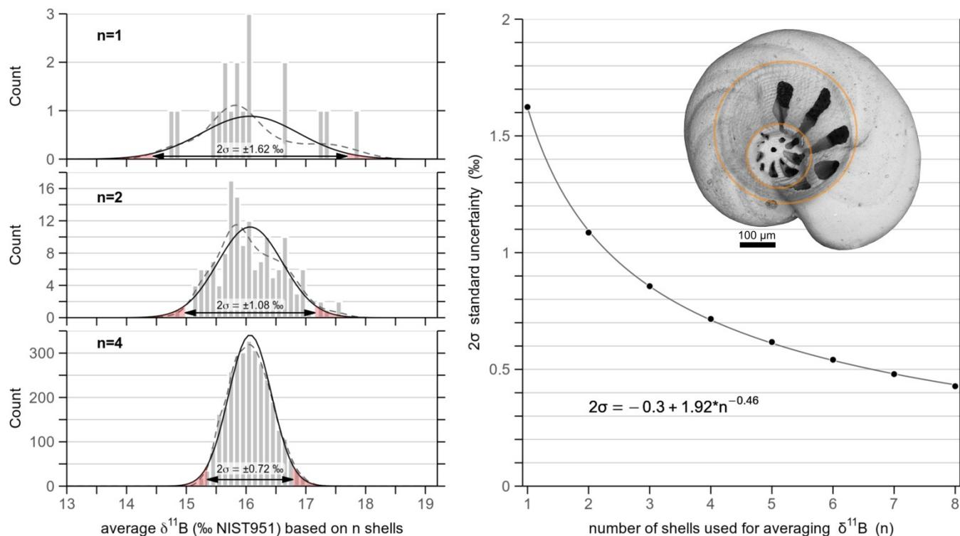
310 Figure 7: Simulation of  $2\sigma$  uncertainty for  $\delta^{11}\text{B}$  using LA-MC-ICPMS in relation to the number of analyzed *C. wuellerstorfi* shells.
