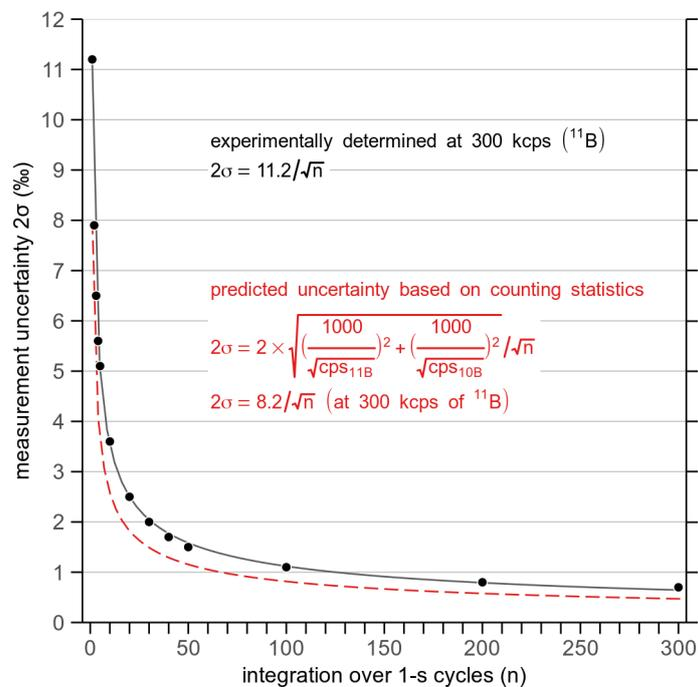
**Figure 3: Measurement uncertainty of  $^{11}\text{B}/^{10}\text{B}$  ( $2\sigma$ ) at count rates of 300,000 cps ( $^{11}\text{B}$ ) as a function of the laser ablation time. The uncertainty of each boron isotope measurement is calculated based on this relationship (black solid line). A major portion (~70 %) of the measurement uncertainty is related to Poisson-distributed counts (red dashed line).**
