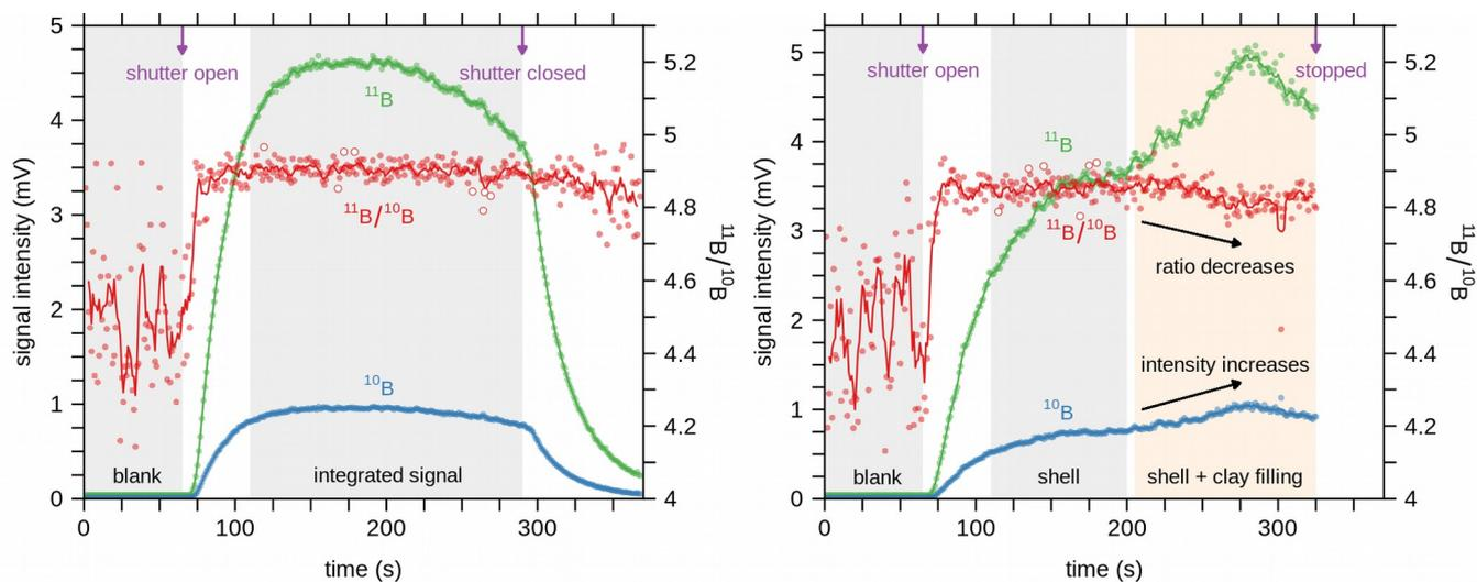
290 **Figure 2:** Left: Typical time-resolved laser ablation analysis for  $^{10}\text{B}$  and  $^{11}\text{B}$  of a *C. wuellerstorfi* shell using Daly detectors, preceded by a  $\sim 60$  s blank measurement. Dots represent 1-s cycles, and lines 5-pt running averages. Open symbols are data that are excluded by the  $2\sigma$  outlier test. Right: Example of a shell that was penetrated by the laser beam, resulting in the ablation of clay infillings.
