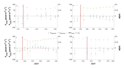
Figure 2: The response of the daily midday medians of NDVI (yellow circles), COS (blue circles) and CO2 (red circles) ecosystem fluxes around the 4 cutting events (a-d) of the grassland. The errorbars depict the respective median absolute deviations. The cuts are marked by a
