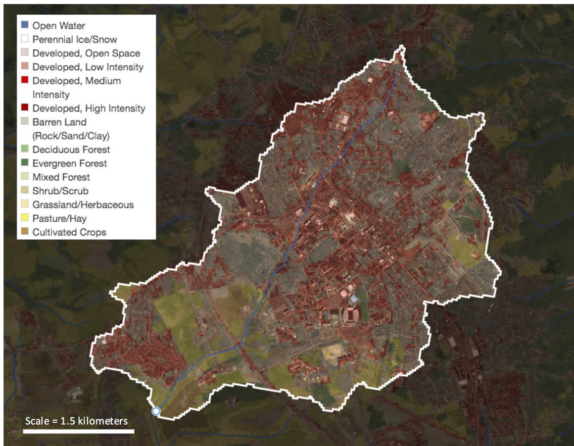
Figure A1. Stroubles Creek watershed and land cover types in the area that drains to the StREAM Lab monitoring site at Bridge 1, Blacksburg, VA, U.S.A. (coordinates in decimal degrees: 37.21013, -80.44511). The nearby weather station that provided light and barometric pressure is just west of the watershed boundary and within the same valley. We created this map using ArcGIS, NHDplus version 2.1, and the U.S. Geological Survey's 2011 National Land Cover Database.
